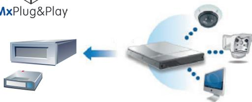
Recordings are directly stored on SnapServer NAS systems over the network. RDX QuikStor removable disk system will be used for data vaulting and data transportation.
