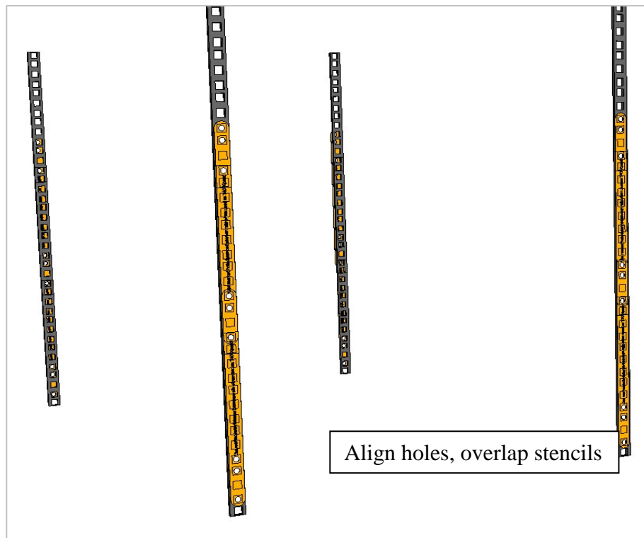
Figure 4. Aligning of the Rack Installation Stencils for systems with more than two units.
